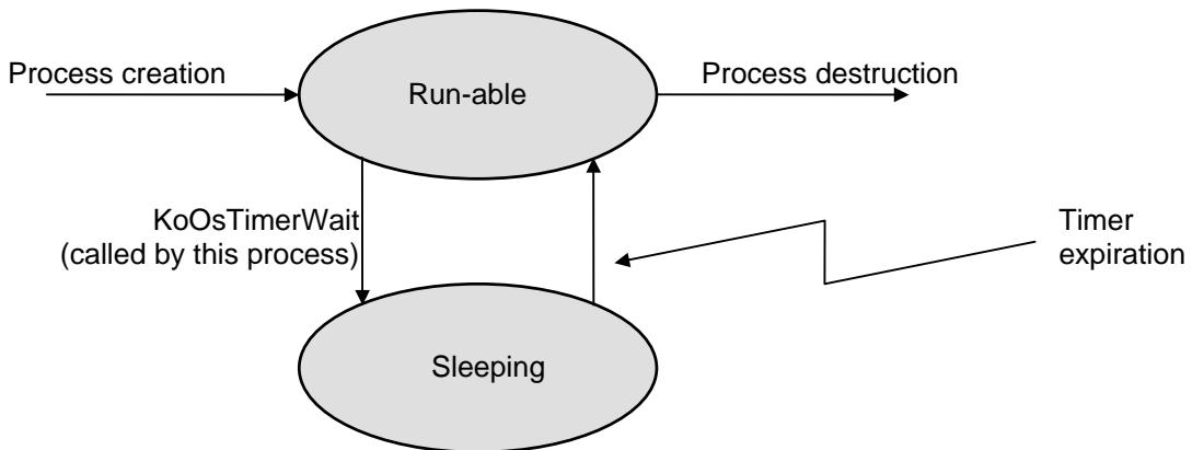
Once the timer is started, the timer will expire (apart from the first time) at a regular interval that you specified as reload value. If you specify the reload value as 0, then the timer will not be reloaded after the first expiration and thus stops. This is the one-shot mode. But there is more : you can influence the timer from the timer function.
