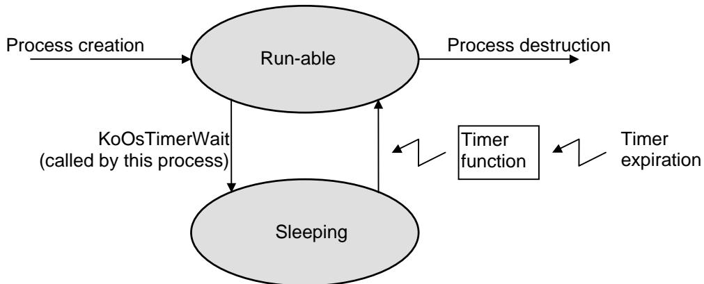
The timer function is called when the timer expires, just before it is reloaded. The timer function receives a pointer to that reload variable and thus can change it to any value it likes. This way you can make enormously complicated timer expiration schemes. You can also change the reload value to 0 which will stop the time gracefully.
