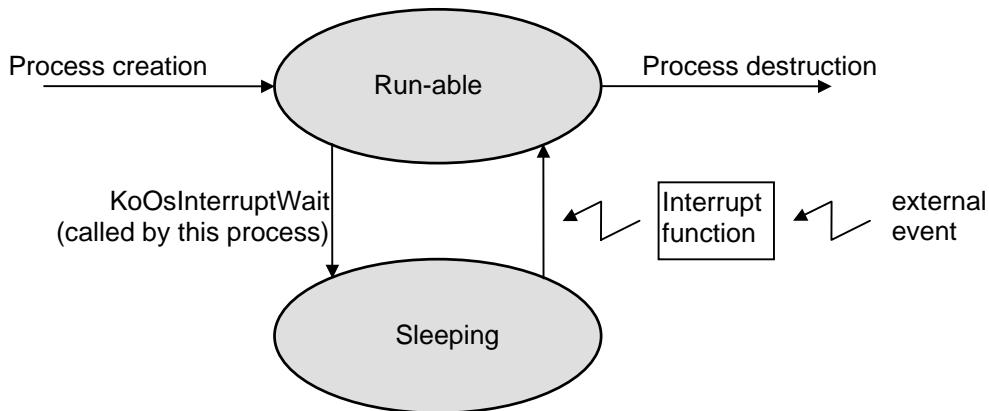
As an example think of a serial port that receives characters from a terminal or keyboard. The serial port receive event can trigger an interrupt routine that stores the received characters in a buffer avoiding an overrun of received characters.
